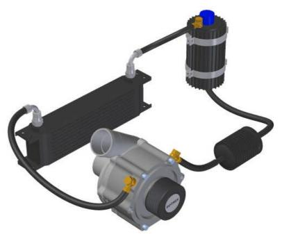
needed for a standard supercharger installation: All hoses, filter, cooler and canister. The oil cooler must be installed where there is good airflow in front of other coolers in the engine compartment
